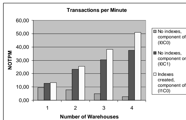
Figure 3. Throughput in a 90 minute test
