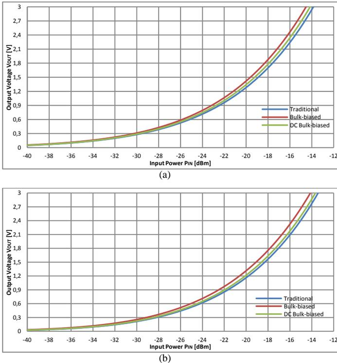
Fig. 6. Output voltage as a function of input power for 0.9 (a) and 2.4GHz (b).
