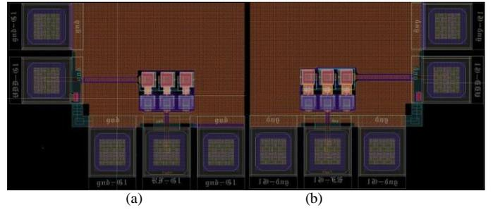
Fig. 7. Traditional (a) and bulk biased (b) voltage multiplier layouts.
