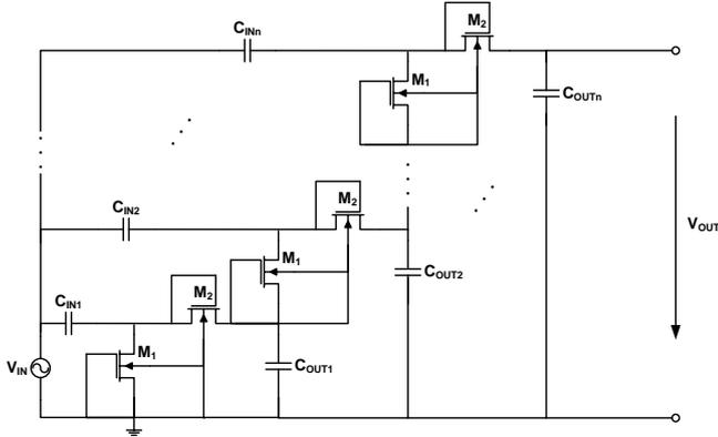
Fig. 4. N-stage DC bulk-biased voltage multiplier architecture.
