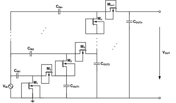
Fig. 3. N-stage gate bulk-biased voltage multiplier architecture.
