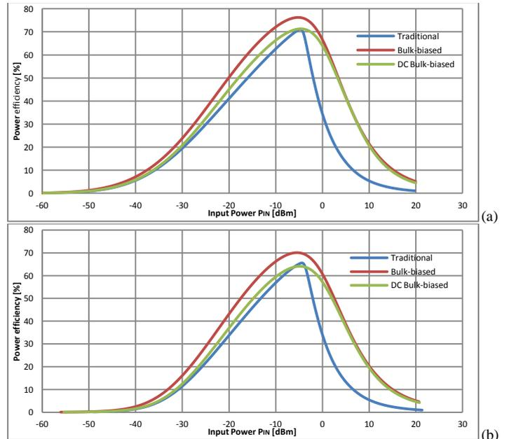
Fig. 5. Power efficiency as a function of input power for  $0.9$  (a) and  $2.4\text{ GHz}$  (b).
