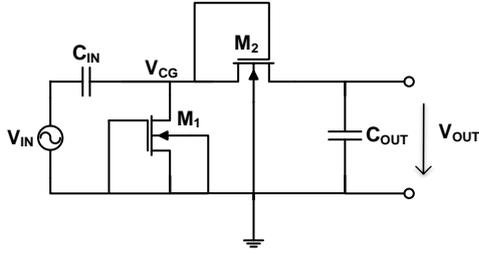
Fig. 1. One-stage traditional voltage multiplier architecture.
