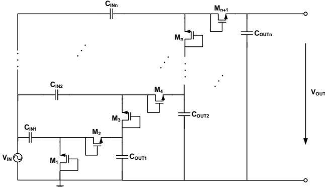
Fig. 2. N-stage traditional voltage multiplier architecture.
